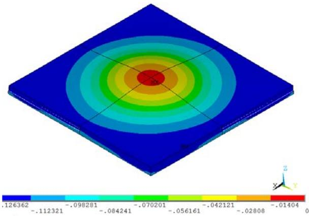
Figure 6: Package warpage data (leg#1) at 25°C
