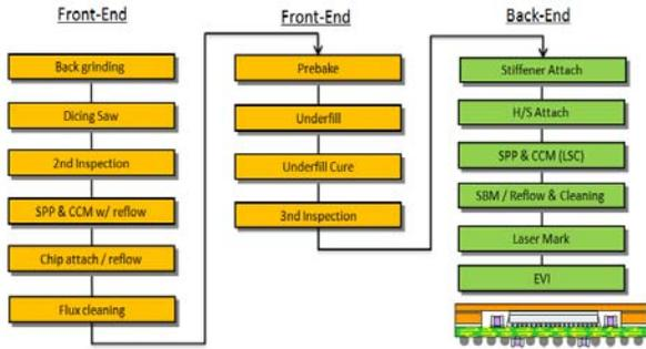
Figure 3: Typical assembly process flow for flip chip BGA
