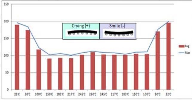
Figure 10: 3<sup>rd</sup> DOE build package warpage data
